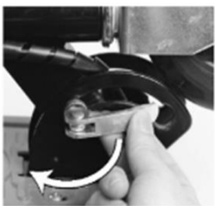
Release the clamp on the hinge joint.
