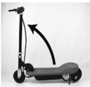
Unfold scooter to fully upright position
