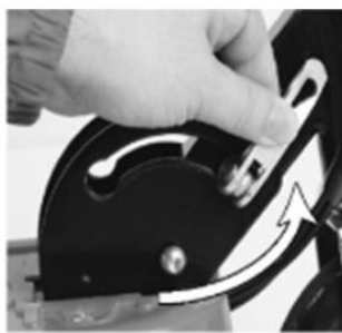
Re-tighten the hinge clamp when steering bar is fully erect.
