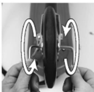
Insert axle bolt through fork and wheel
