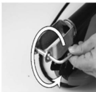
Release the axle bolt with left turn
