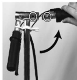
Align Handle with T-Bar: hole in T-Bar aligns with tab on inner end of handle
